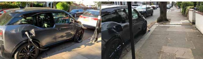
A pair of photos showing how the owner of this e-vehicle uses an adapted lamp column to charge the battery when they can get access to the kerbside in that location, and uses a trailing cable from their home when they cannot park near the lamp column.
