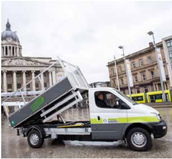
Figure 20 – Battery-electric cage tippers used for refuse collection in Nottingham (Image source: Nottingham City Council)
